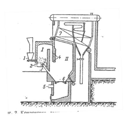
To burn fine residual particles of low-reactive fuels. No cooling tubes in these figures!
