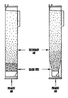
"The Foster Wheeler process is characterized by the presence of a pronounced bed in the bottom few feet of the furnace and a relatively solids-lean freeboard above it.
