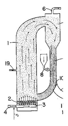
Lewis 1941-44 was the first to propose a CFB reactor "Reaction between solids and gases"
